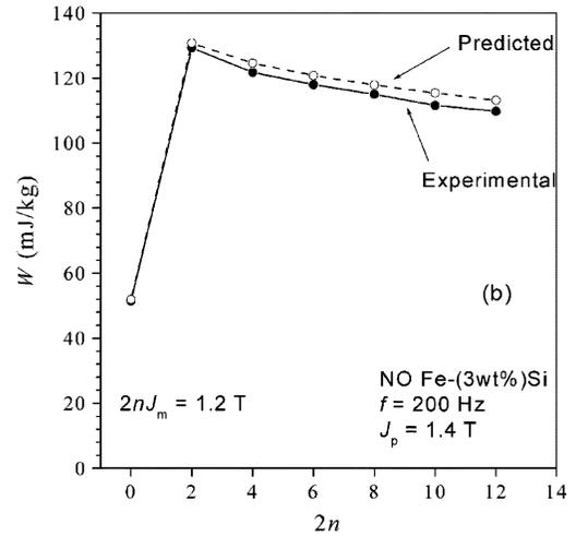
Fig. 6. Evolution of the energy loss with the number of minor loops in a nonoriented Fe–3wt%Si lamination under controlled constant magnetization rate  $|\dot{J}(t)| = 4f(J_p + 2J_m)$ , with  $J_p = 1.4$  T and  $2nJ_m = 1.2$  T. Examples of associated composite hysteresis loops (for  $n = 2$  and  $n = 6$ ) are shown in Fig. 3. The total loss prediction is made for  $f = 50$  Hz and  $f = 200$  Hz by means of (26), specific to this case through (27)–(29).
