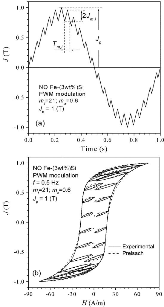
Fig. 7. Magnetic polarization  $J(t)$  and hysteresis loop behavior with a two-level PWM supply. This example is characterized by modulation frequency ratio  $m_f = 21$  and modulation index  $m_a = 0.6$ . Peak polarization value  $J_p = 1$  T. Corresponding experimental (solid lines) and reconstructed (dashed lines) quasi-static hysteresis loops in nonoriented Fe-(3 wt%)Si laminations (thickness 0.34 mm) are shown in (b). The loop reconstruction has been made as in Fig. 3.
