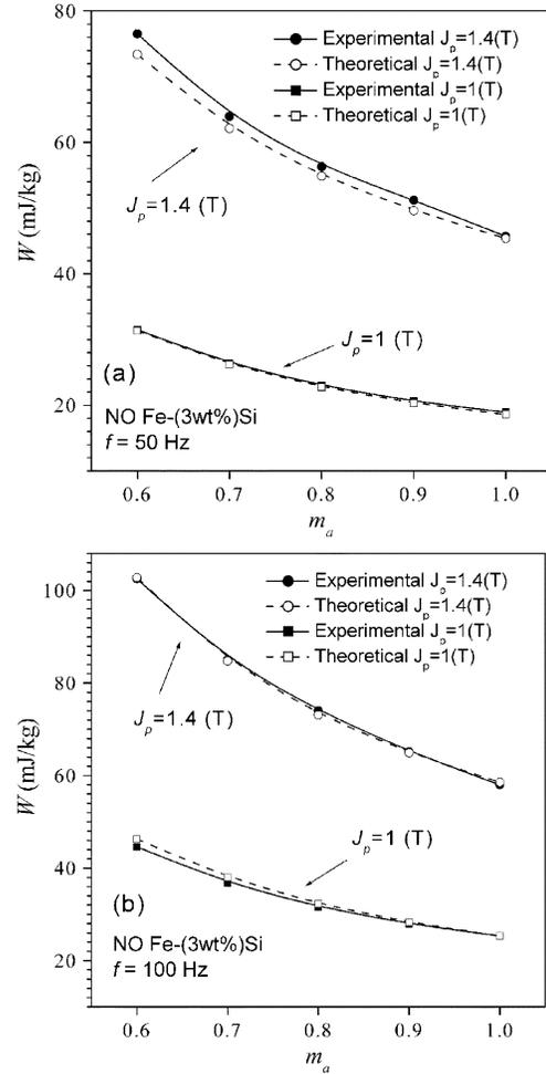
Fig. 8. Experimental and predicted energy loss behavior under two-level PWM supply with modulation frequency ratio  $m_f = 21$ , modulation index  $m_a$  varying between 0.6 and 1, and frequency (a)  $f = 50$  Hz and (b)  $f = 100$  Hz. An example of associated quasi-static composite hysteresis loop ( $m_a = 0.6$ ,  $J_p = 1$  T) is shown in Fig. 7(b). The total loss prediction is based, as always, on (26), formulated in terms of modulation parameters through (32), (33), and (36).
