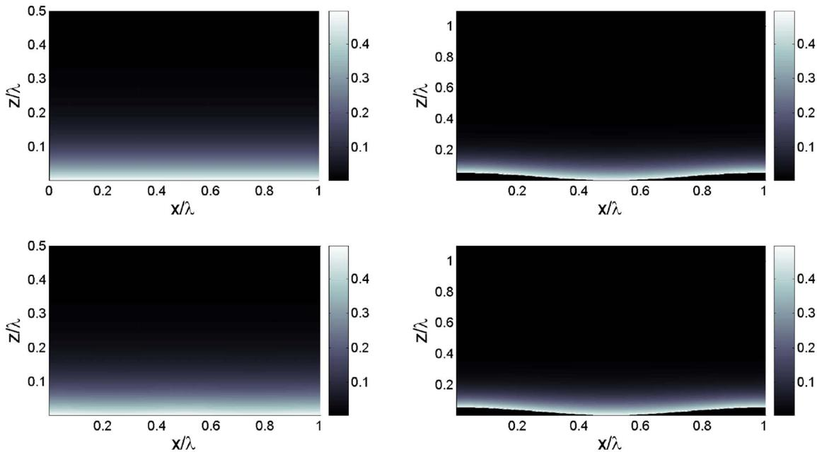
FIG. 2. (Color online) Distribution of the elastic energy density Eq. (3) when  $qA = 0.15$ . Upper left: case 1 [flat surface with approximate boundary conditions (BCs)]; upper right: case 3 (exact surface with approximate BCs); lower left: case 2 (flat surface with exact BCs); lower right: case 4 (exact solution).
