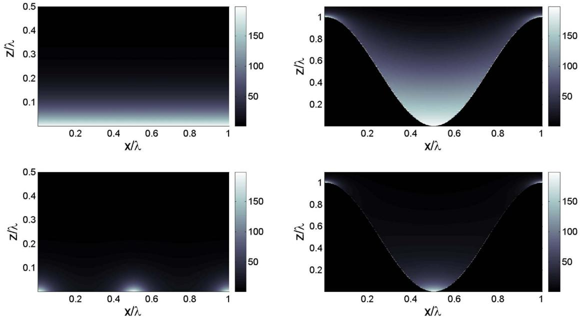
FIG. 3. (Color online) Distribution of the elastic energy density Eq. (3) when  $qA=3.0$ . Upper left: case 1 (flat surface with approximate BCs); upper right: case 3 (exact surface with approximate BCs); lower left: case 2 (flat surface with exact BCs); lower right: case 4 (exact solution).
