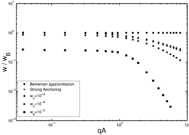
FIG. 5. Equivalent anchoring energy normalized to the value calculated by Berreman's analytical solution Eq. (1) as a function of  $qA$ . Comparison of the results with different anchoring strengths  $w_e = \infty$ ,  $2\pi \times 10^{-3}$ ,  $2\pi \times 10^{-4}$ , and  $2\pi \times 10^{-5}$ .
