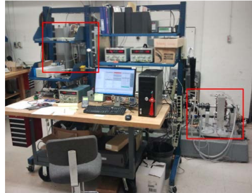
Figure 14. Setup #1, used for the IPM and the SPM machines. The dSPACE 1103 PPC host computer is on the desk. The machine under test is in the red square at the bottom right corner, connected to an induction machine dynamometer via a torque-meter (not visible). Power converters are in the other square on the left hand corner.
