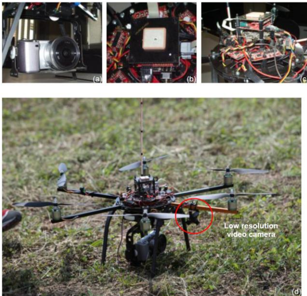
Figure 2. The digital camera Sony NEX-5 (a), The Ublox GPS receiver antenna (b), the electronic control unit (c). In (d) from the highest to the lowest part: BL, FC, NC, MK3Mag, MKGPS, and the Hexakopter by Mikrokopter
